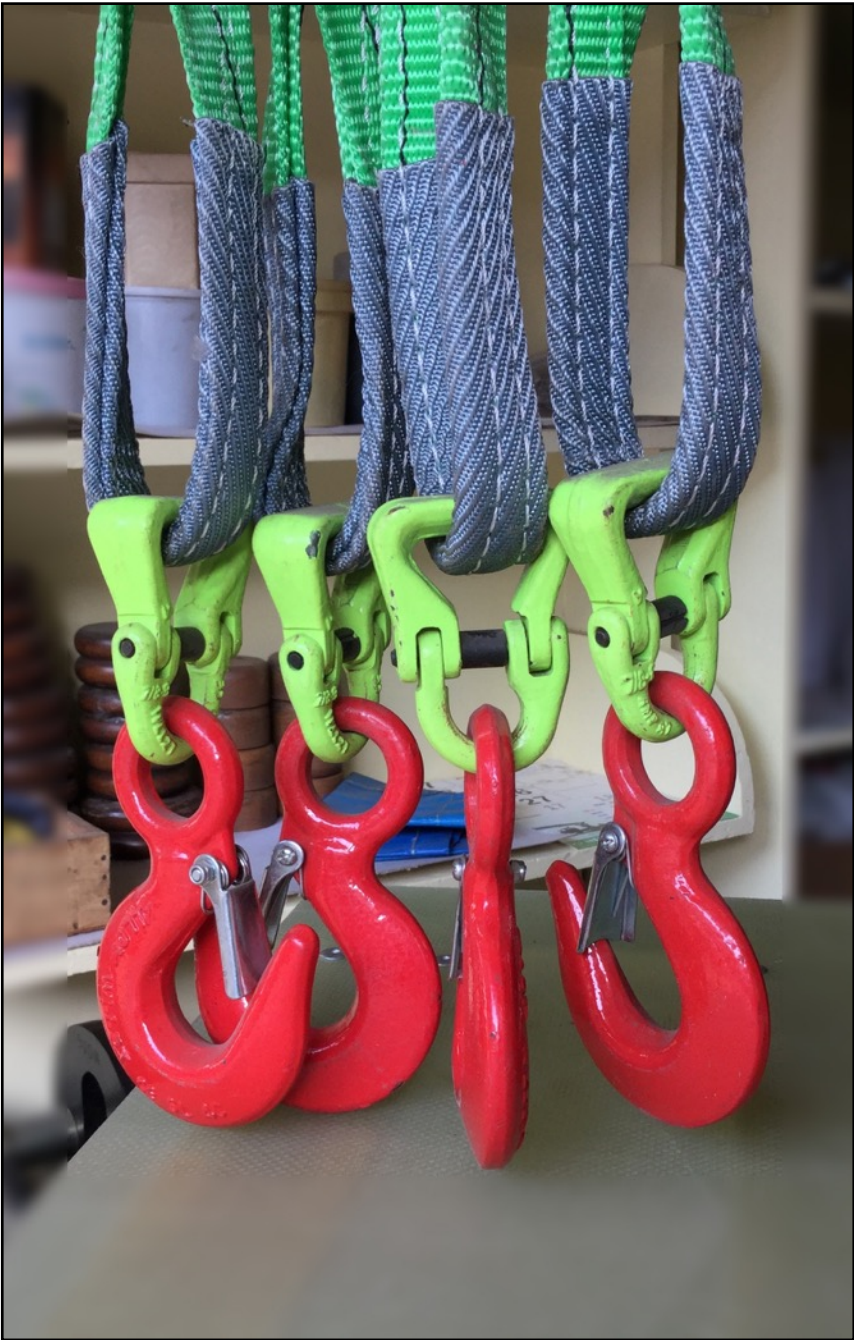
FIG 1: WEB SLING CONNECTOR USED FOR COUPLING WEB SLING WITH EYE HOOK
