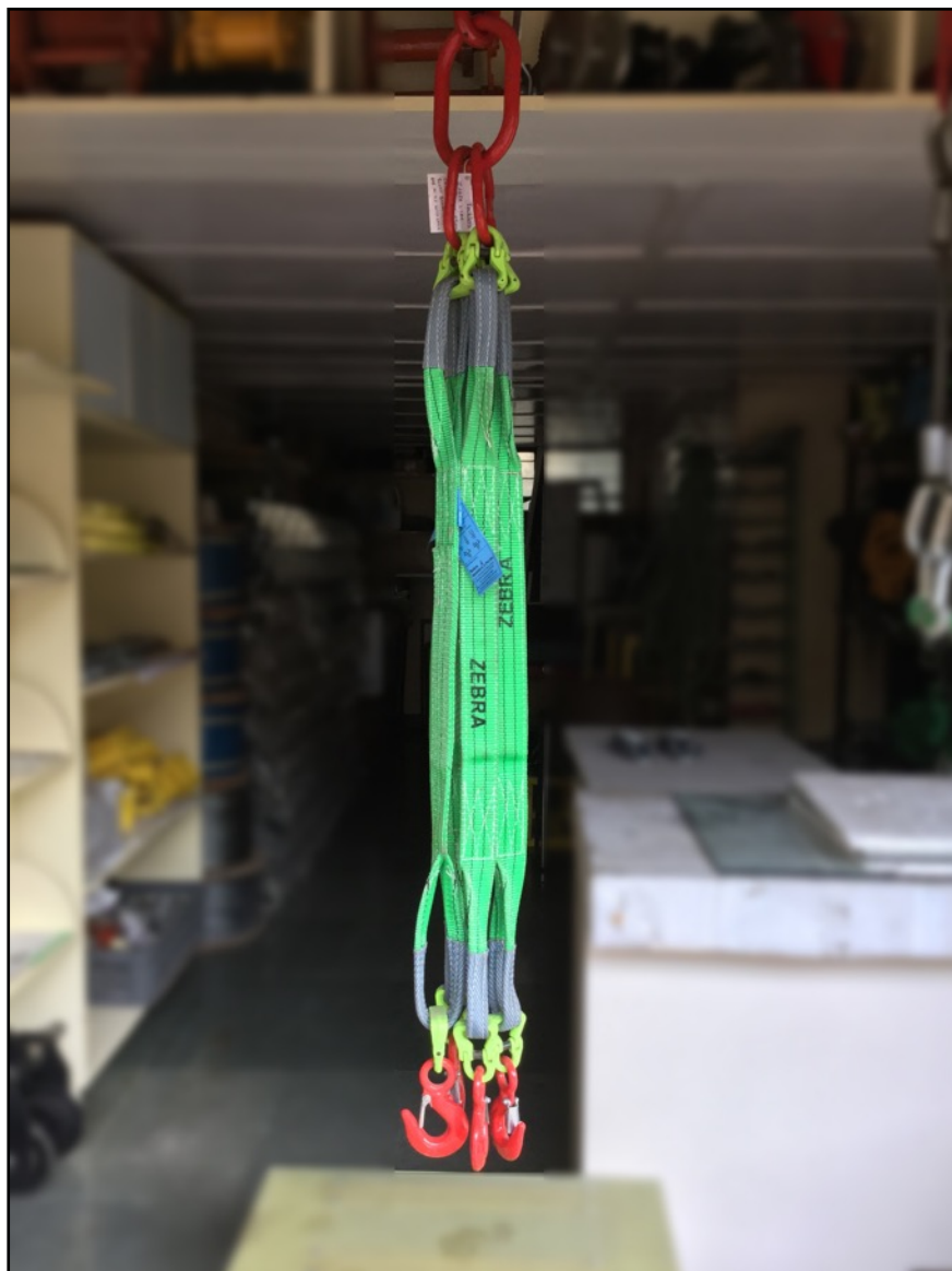
FOUR LEG SLING MADE WITH 2 TONS DUPLEX FLAT WEBBING SLING WITH LOOPS AT BOTH ENDS
