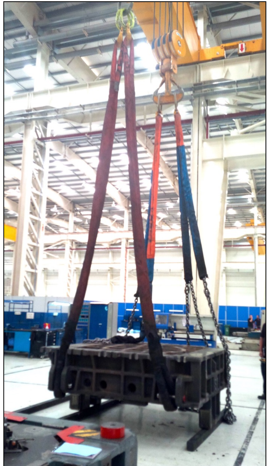
FIG 4: TWO DOUBLE LEGGED COMBINATION SLING WITH CHAIN AND POLYESTER USED FOR DIE LIFTING
