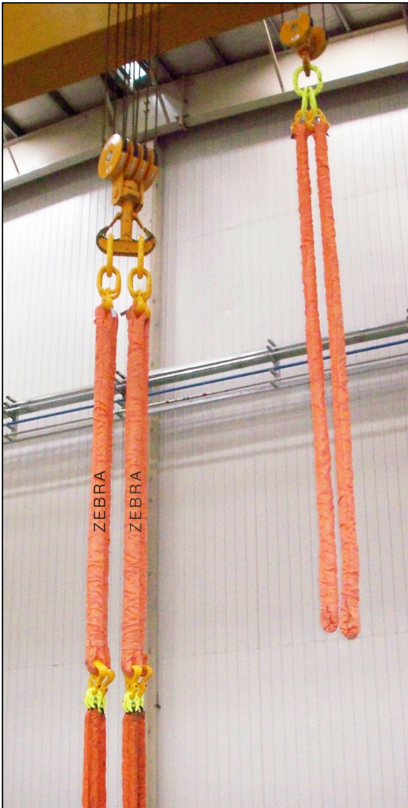
FIG 3: TWO DOUBLE LEGGED DUPLO ROUND SLING ASSEMBLIES - 50 TONS CAPACITY
